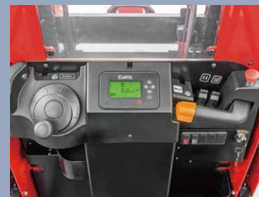
The FREE accelerator lever with sensor switch, as standard configuration, can prevent mis-operation during the work
