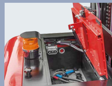
The rear hood can be removed easily to facilitate maintenance work on parts such as hydraulic unit, electronic control system and the motor
